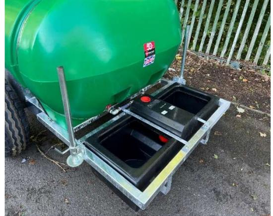
**CHASSIS** Constructed from 5mm pressed steel section fully welded with a 100 x 50 R.S.C 'A' frame drawbar and a front standplate.
