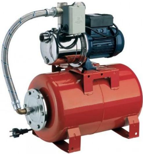
Hydropress pumps are Ebara self-priming pumps fitted with a pressure switch and expansion vessel. They can draw water from a storage tank or well up to 8 metres deep when fitted with the optional foot valve.
