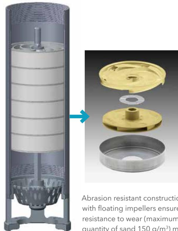
Abrasion resistant construction combined with floating impellers ensures optimum resistance to wear (maximum permissible quantity of sand 150 g/m<sup>3</sup>) making this one of the best pumps on the market for sand handling capabilities.
